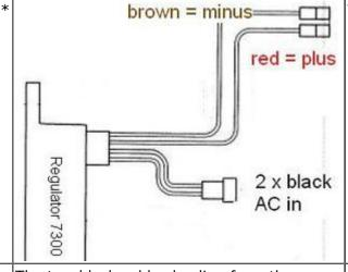
The new regulator/rectifier has 4 wires
