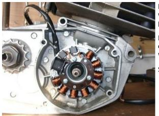
Put the stator coil back onto the plate, take care not the damage the wires. The stator has to snap in rather sharply. If it sets soft, you have probably jammed a wire underneath!
