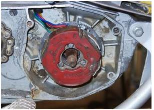
Remove all cables that goes to the old ignition coil and to the ULO-box and take off these parts.
