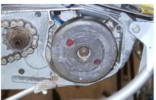
Make sure your motorcycle rests securely on her stand, preferably on an elevated work bench and that you have good access to the generator side of the engine. Note that you will install a 12 volts system, so you will need to replace all lightbulbs to 12 volt ones.
